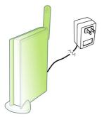
For initial setup, plug your desktop or notebook computer directly into the LAN Port #1 with the included CAT5 patch cable. Please make sure that your computer LAN setting is DHCP or 192.168.62 x. Submask: 255.255.255.50.
